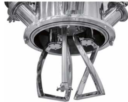
図3 攪拌部形状 Fig.3 Mixing part shape
