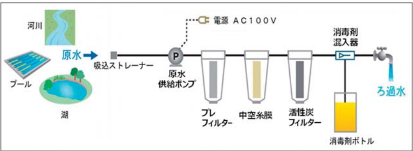
図2 処理フロー Fig.2 Process flow diagram of MIZU cube
