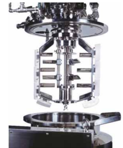
図8 アチホミキサー®攪拌部 Fig.8 Mixing section of AGI HOMO MIXER
