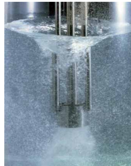
図6 逆転運転時の液の動き Fig.6 Liquid flow of reverse operation
