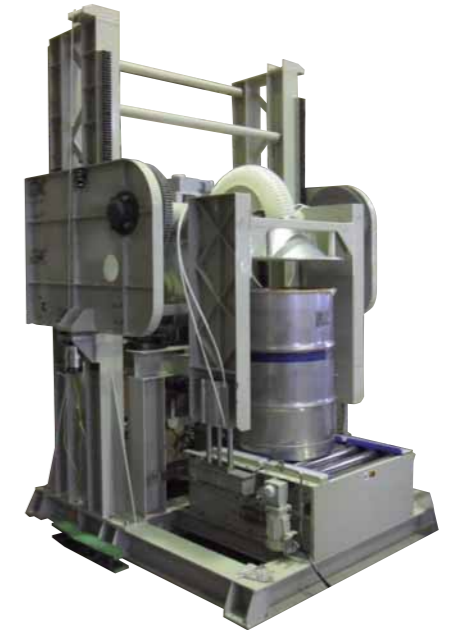
図2 ドラム反転投入機実機写真(A社向け) Fig.2 Photo of actual drum reversing and feeding device (For company A)
