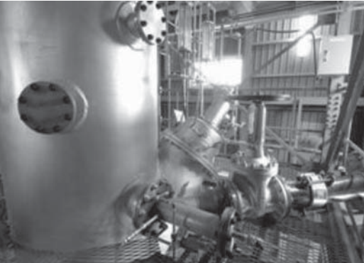
図6 過給式流動炉(汚泥投入部) Fig.6 Photo of Fluidized Bed Incinerator with turbocharger
