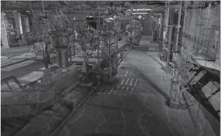
図3 AS BUILT SCAN Fig.3 AS BUILT SCAN
