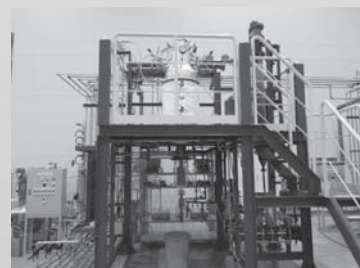
図1 液中燃烧炉 Fig.1 Submerged Combustion System
