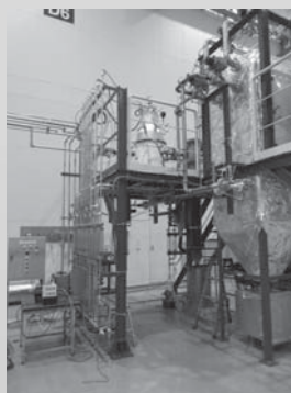
図2 粉体回収装置 Fig.2 Ultrafine Particle Recovery System
