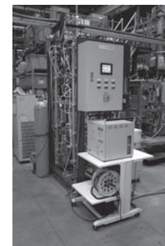
図5 PSA 型溶剤回収装置 Fig.5 Pressure Swing Adsorption
