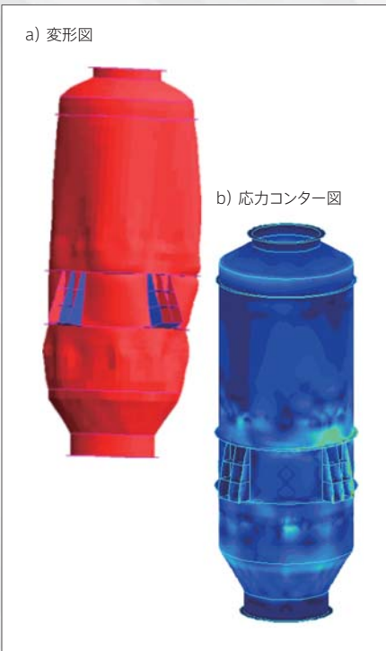
図3 燃烧炉解析結果 Fig3 Analysis results of combustion furnace
