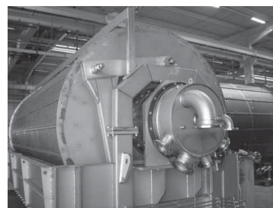
Fig.1 BOKELA drum filter (40m²)
