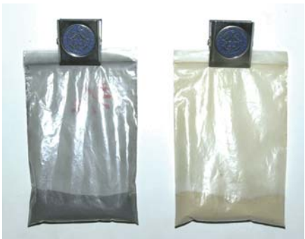
図4 石炭の常圧FBCとPFBCでの灰の比較 左：常圧、右：加圧 Fig.4 Photograph of ash produced by FBC and PFBC. Left: Atmospheric condition. Right: Pressurized condition (0.8MPa).
