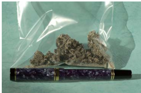
図5 石炭の場合に流動層内で生じたアグロメレーション Fig.5 Photograph of agglomerate produced in the fluidized bed at pressurized condition.
