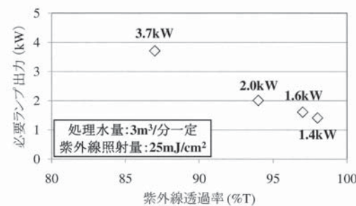
図8 紫外線透過率と必要ランプ出力の関係 Fig.8 Relation between UV transmittance and requisite lamp output
