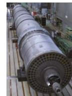
Steam tube dryer (large-scale industrial dryer)
