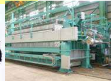
Filter press (dewatering machine)
